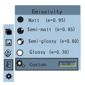
As shown in the figure, press " MENU/  $\circlearrowleft$  " key to enter the main menu and select "  $\mathcal{E}$  "(emissivity) option and press "  $\blacktriangleright$  " key to enter the emissivity list.
