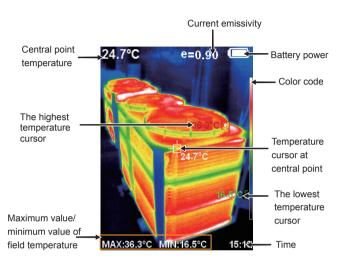
Color code: used to mark the color corresponding to the relative temperature from low to high in the field of version.
